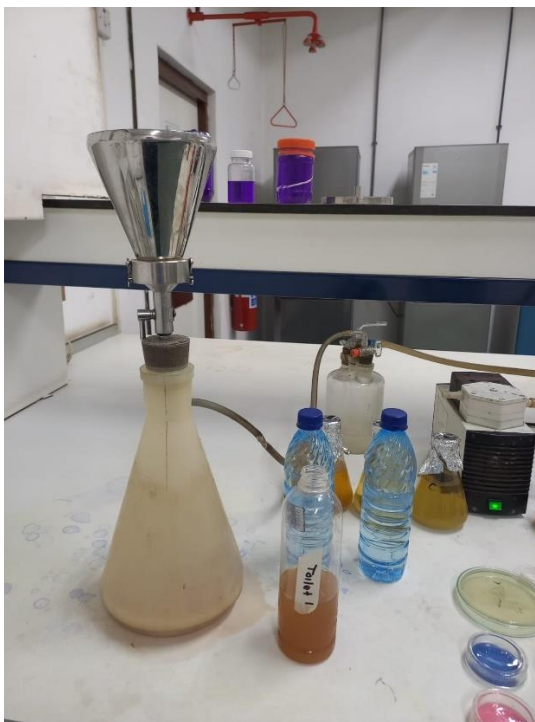
Figure 9. Filtering the urine sample using a suction pump in the laboratory of the University of Zambia.
