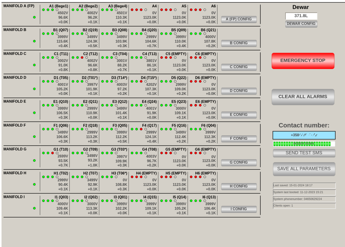
FIGURE 21 The new main page of the HMI provides a comprehensive overview of the system’s status. It shows, for example, the detector temperatures, voltages, and active channels.
