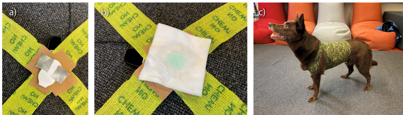
Fig. 1. (a) Preparation phase: electrodes were attached to self-adhesive elastic bandage and protected with cover and adhesive tape. (b) To optimize the connection, saline solution and conductive ultrasound transmission gel (AquaSonic100, Parker Laboratories Inc., Fairfield, CA, USA) were applied to the cotton sheet with electrode location. (c) To keep the electrodes firmly in contact with the skin, a self-adhesive elastic bandage was applied carefully around the dog chest on top of the electrodes.
