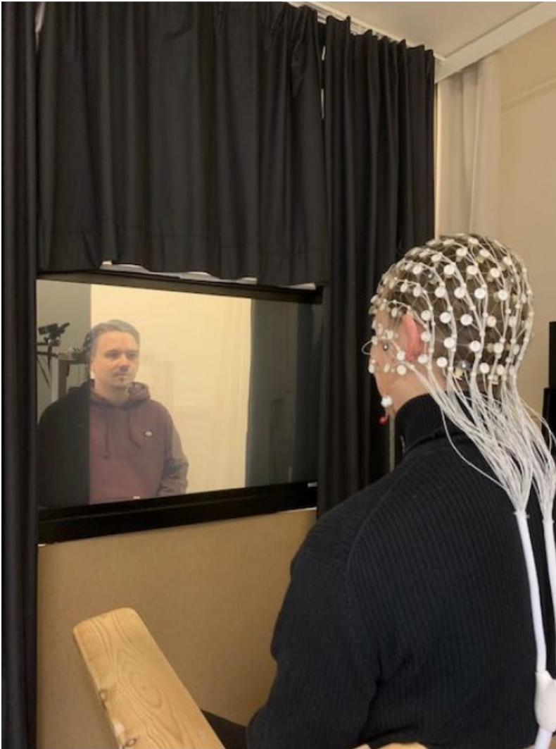
Figure 1. The setup for the experiment: participant and face model are divided by a 44cm x 53cm liquid crystal screen that can turn either opaque or transparent within 1ms. During the actual experiment lights were turned off on the participant's side.
