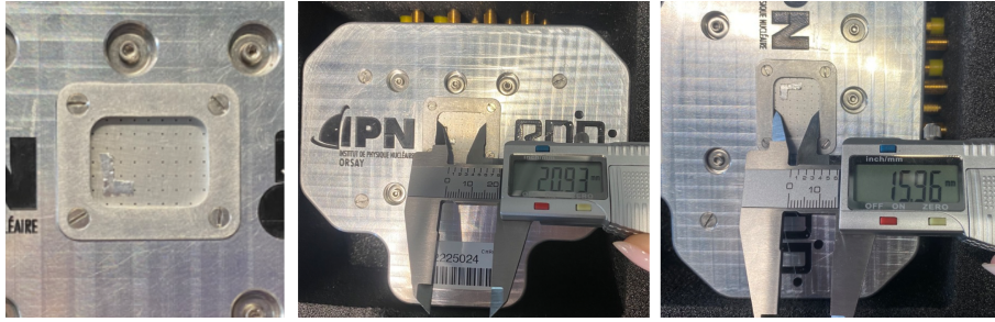
Figure 6. The properties of the grid that was use in front of the diode. On the left figure the L shaped tin foil shielding element used during measurement is presented. In the figures in the middle and right we can see that the grid is slightly smaller than the diode.
