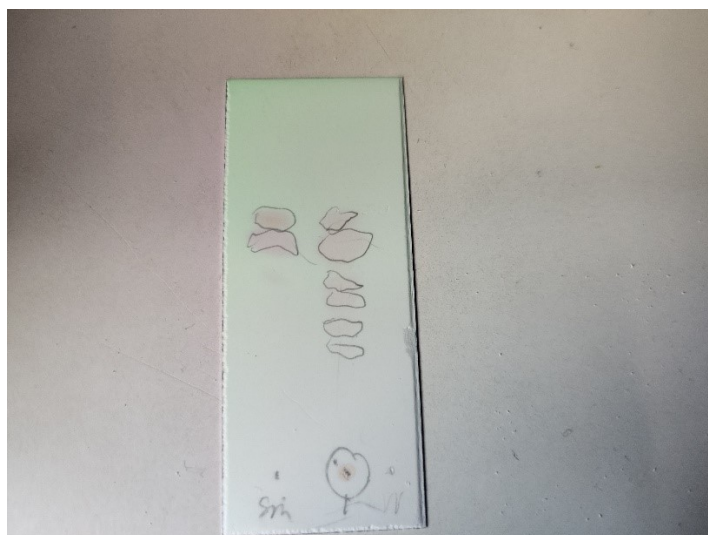
Figure 45. TLC plate of reaction TIM-208.1 (the same TLC pattern was observed for all other reactions except TIM-215 and TIM-217). The left-side spots represent to the starting material, while the right-side spots represent reaction solution prior to chromatographic purification.
