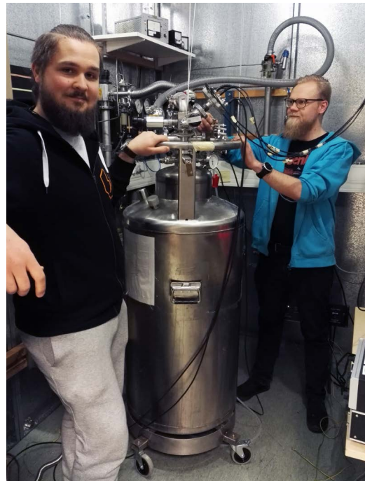
↑ Dilution refrigerators are used to cool samples down to 50 mK.
