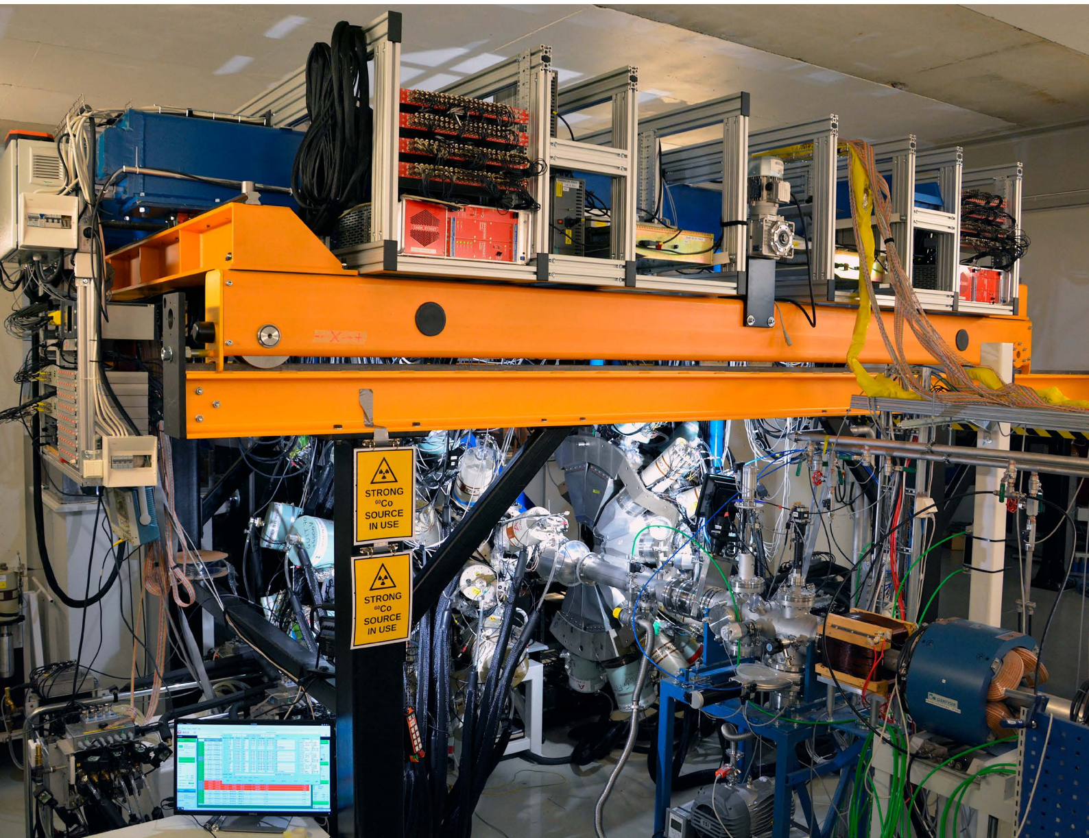
↑ The JUROGAM3 array of germanium detectors installed at the target position of the MARA separator.
