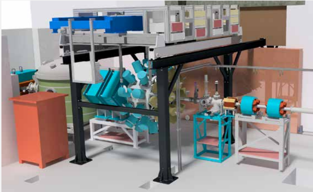
→ Figure 3: A schematic view of the JUROGAM3 array of germanium detectors installed at the target position of the MARA separator.
