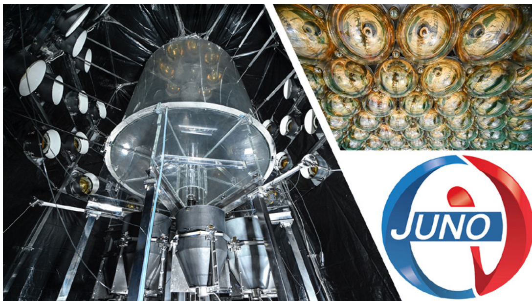
↑ Figure 1. Left – JUNO-OSIRIS setup – the standalone radiopurity detector for liquid scintillator screening before filling the Central Detector. Right – a small section of the JUNO Central Detector's 45 thousand PMT light sensors.
