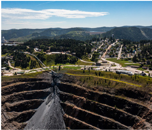
← Figure 2. Top – bird's view of Lead, South Dakota and the decommissioned Homestake Mine. The 800,000 tons of excavated rock from the DUNE caverns were transported with a 1.3 km-long conveyor belt and deposited in the open pit. Bottom – one of the caverns ready to house DUNE liquid argon cryostats.
