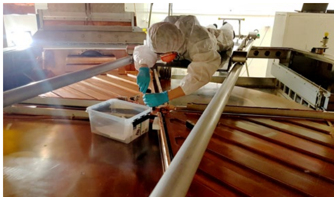
↑ Figure 3: Taneli Kalvas installing the new central region of the K130 cyclotron.
