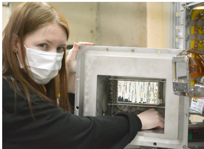
↑ Figure 2: Henna Joukainen installing the scintillator detector in the focal plane vacuum chamber of MARA.
