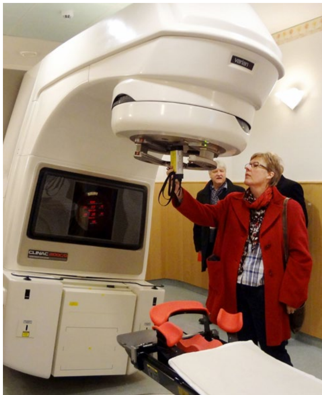
↑ Figure 4: Jaana Kumpulainen checking the residual activity in an electron accelerator used for radiation therapy.
