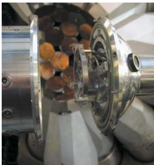
Fig. 4. The plunger device employed with JUROGAM at RITU for RDDS lifetime measurements.
