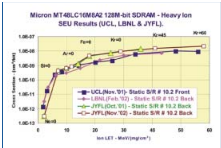
Fig. 5. Comparison of the SEU data taken in the three laboratories: UCL, LBNL and JYFL (private comm. with Mr. Reno Harboe-Sørensen, ESA/ESTEC).
