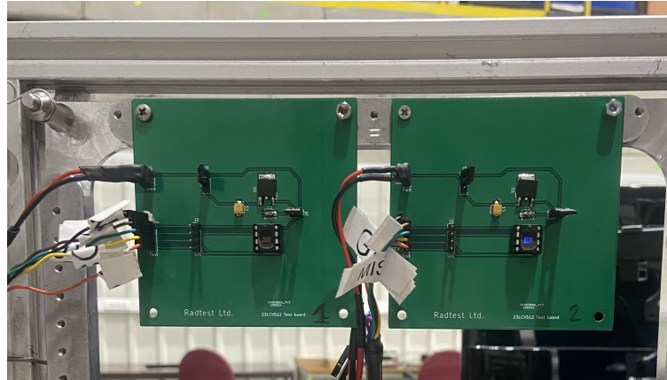
Figure 9. The board connections for 23LCV512 inside the vacuum.
