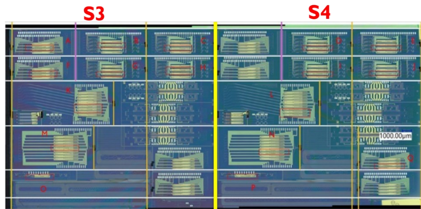
Figure 18: 1 st batch die of samples S3 and S4 with named (red) and diced (yellow)
