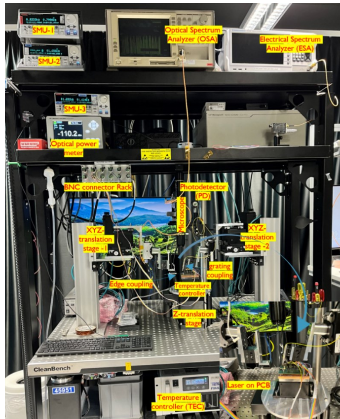
Figure 24: The Experimental setup used for the characterization of lasers
