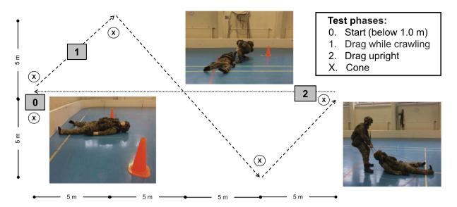
Figure 1. Casualty emergency evacuation test procedure.
