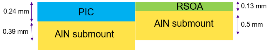
Figure 5: Assembly design with AlN submounts as heat dissipation platforms
