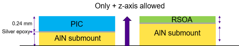
Figure 9: Thickness matching limiting moving in the negative z-axis direction
