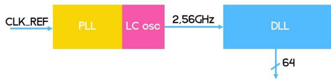
Figure 1.5 TDC architecture based on a PLL, LC oscillator and DLL
