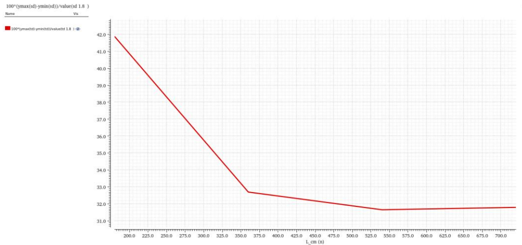
Figure 3.8 Delay variation of Maneatis cell (180nm) due to VDD variation of \pm 10\% (1.62V...1.98V) vs tail current source channel length
