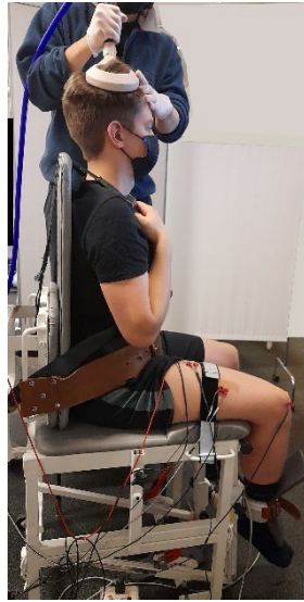
Figure 9 Set up of the Participant position in all Studies and testing sessions. The TMS coil was placed above the M1 leg representation. EMG was placed over RF and vastus lateralis, and the ground electrode was placed on the patella. The torso and leg were strapped to avoid any undesired hip flexion, hip abduction or adduction.
