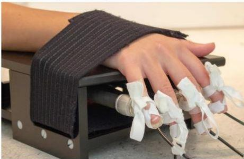
FIGURE 8. Four-finger pneumatic actuator and tactile stimulator.
