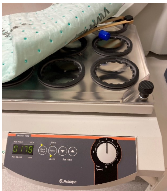
Picture 2. Mixing the covered test tube with the level shaker.
