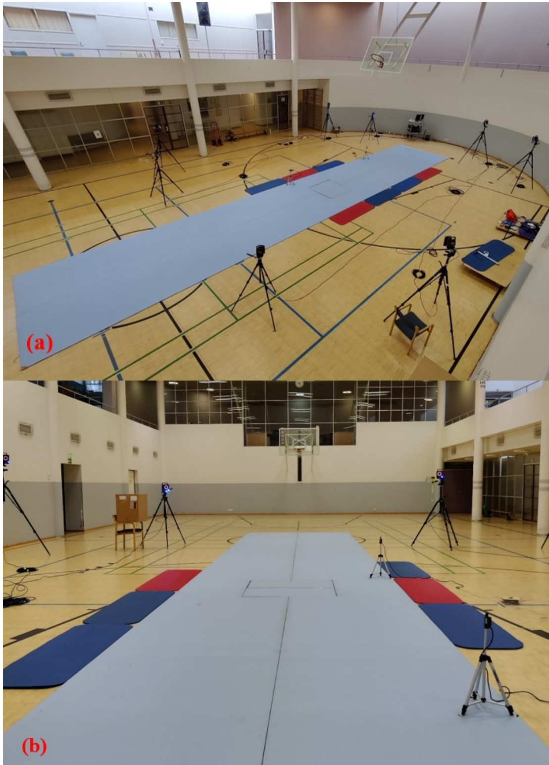
FIGURE 10. Set-up of the running trials. a) Eight cameras (Vicon T-series) were positioned around two synchronized force plates (AMTI BP6001200-2K) embedded in the surface of the runway. b) Two photocells (Newtest Powertimer) were placed 5 metres apart and centred on the force plates within the motion capture space.
