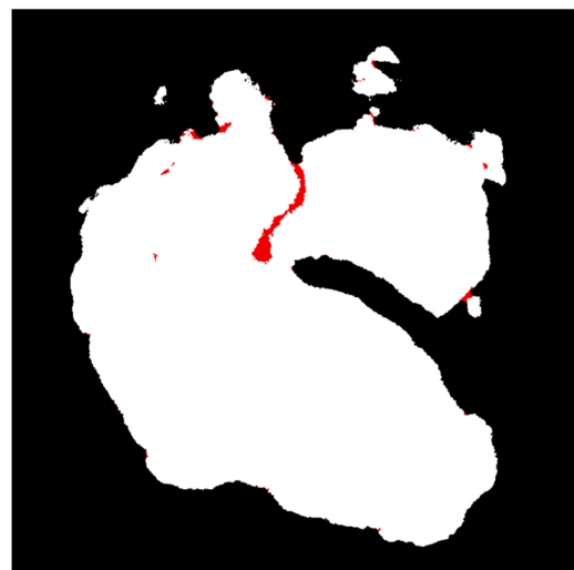
Fig. 2. Segmented 2D image of a soil aggregate. Pores are shown in red, solids in white and exterior of the aggregate in black.
