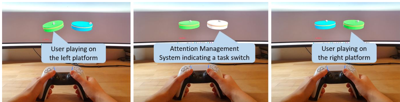
Figure 1: We devised a balancing game to study AI-based assistance that helps users in task switching. The game consists of two platforms where only one can be actively controlled at a time. The goal is to balance the balls as long as possible on top of their platforms. To support users, we implemented a reinforcement learning (RL) based attention management system (AMS) that automatically switches between the platforms (indicated by a sound and a change of the active platform's color). The AMS agent has full access to the states of the subtasks and learns a policy to switch in a way that humans' game scores increase.
