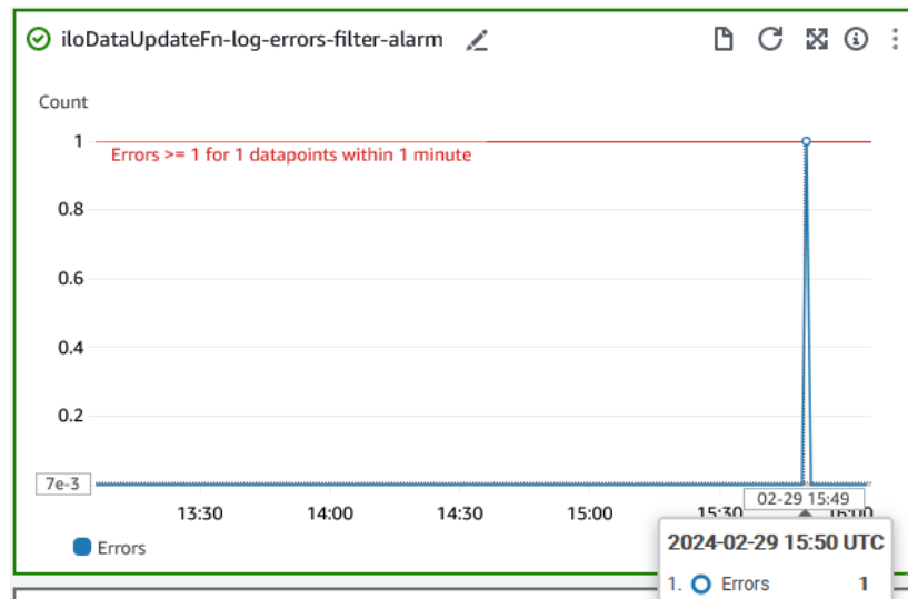
Figure 8. AlarmWidget displaying the error metrics, threshold and activations of the target alarm.
