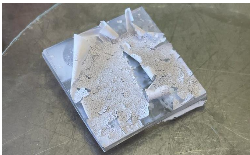
Figure 42. The partially peeled layer of the FTO film in the synthesis of EBP-073.
