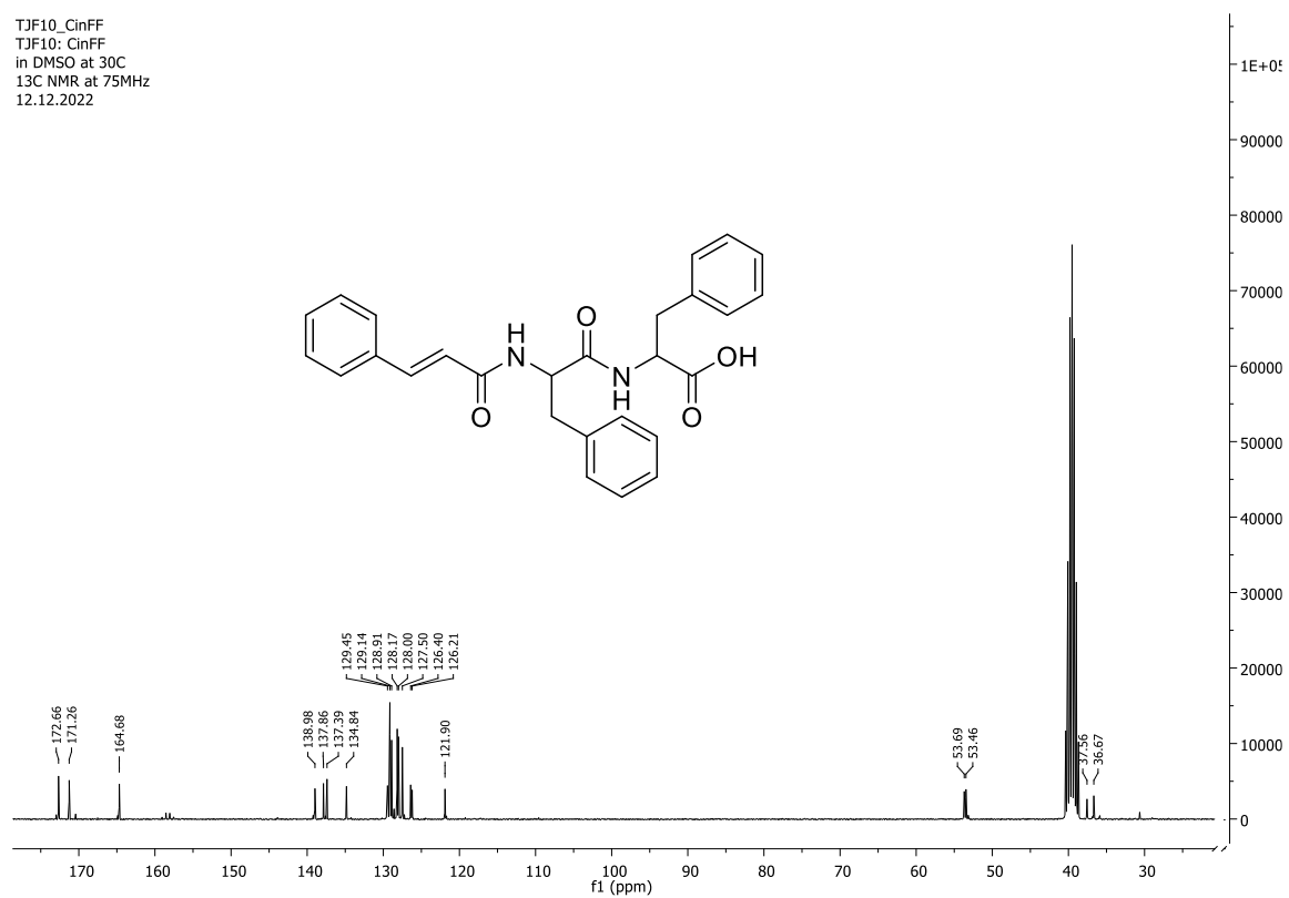
Figure 24. 13 C NMR (75 MHz, d 6 -DMSO) spectrum of CinFFCOOH.
