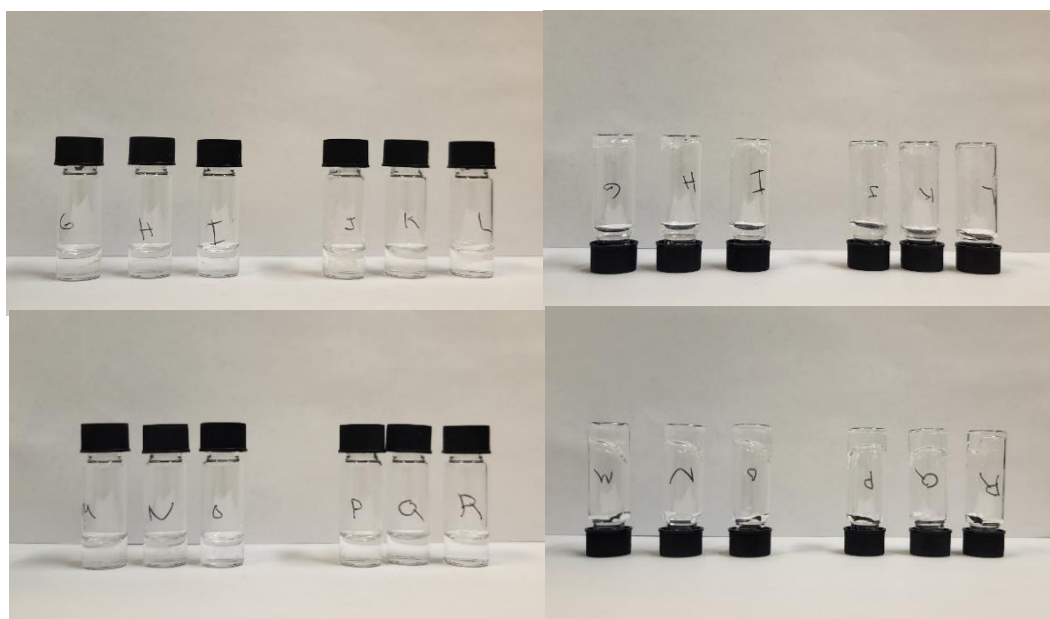
Figure 27. The vial inversion test of samples G-I, J-L, M-O and P-R at day 1.
