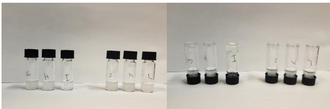
Figure 28. The vial inversion test of samples G-I and J-L after heating and cooling (day 1).
