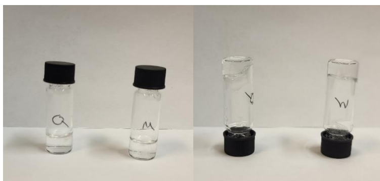
Figure 29. The vial inversion test of samples Q and M demonstrates that the gelation ability of the samples is not altered after re heating and cooling (thermoreversible gels).
