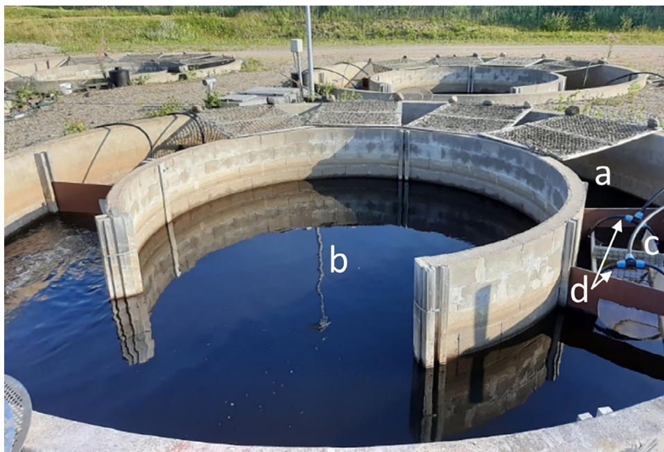
FIGURE 1 Seminatural outdoor stream, consisting of a shallow predator-free section (a, covered section in the back) and a deeper pool section (b, front and middle) containing predatory pike in half of the streams. The sections were separated by a mesh grid wall (c) on either side of the shallow section that allowed salmon to pass, but restricted pike to the pool section. On each side of each mesh grid wall, two passive integrated transponder (PIT) antennas (d) recorded the identity of bypassing fish. Photo credit: Pekka Hyvärinen.
