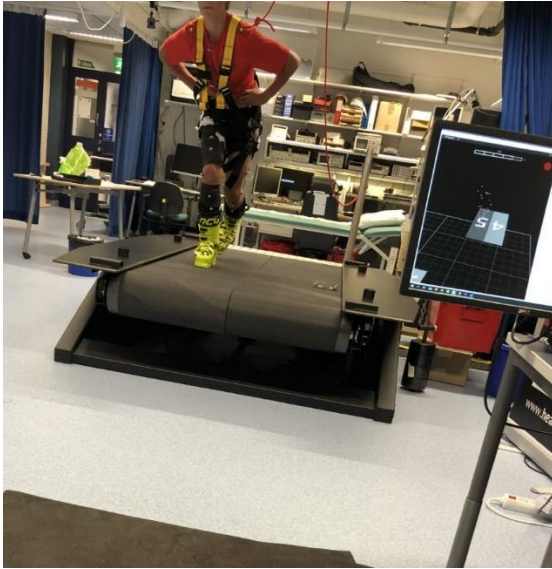
Figure 6. Instrumented treadmill (Motek) and the test position in anterior-posterior direction
