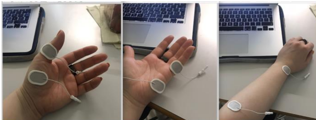
FIGURE 6: sEMG sites (different electrodes). Left to right: APB, ADM, ED.
