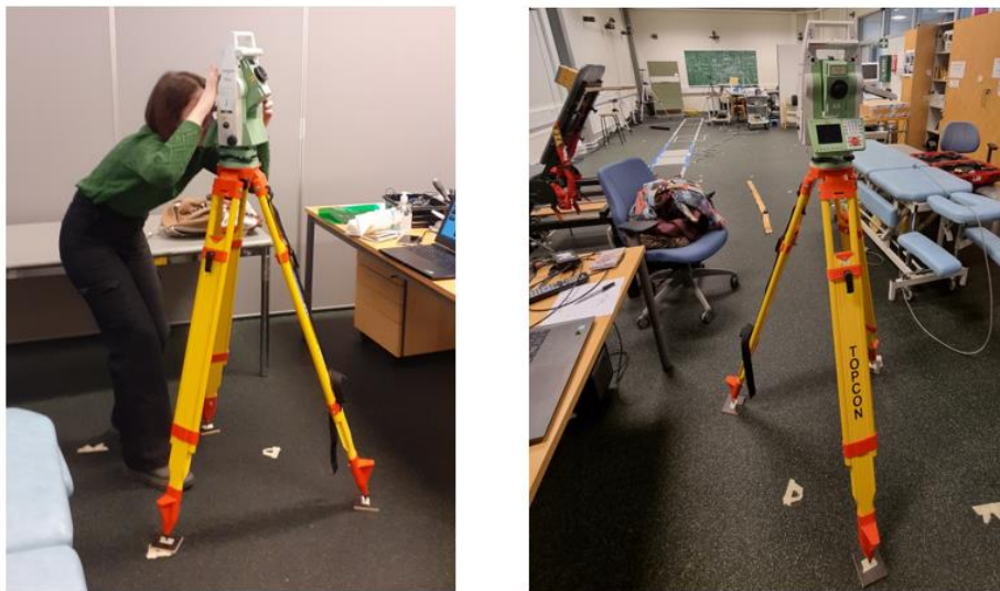
FIGURE 18. The coordinates of the marked points in the capture volume were measured with a tacheometer for the laboratory volume calculation.
