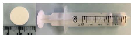
Fig. 1. SLS 3D printed 5 mm (diam. 16.5 mm) 3D-Thiol filter (left) and filter placed in a syringe (right).
