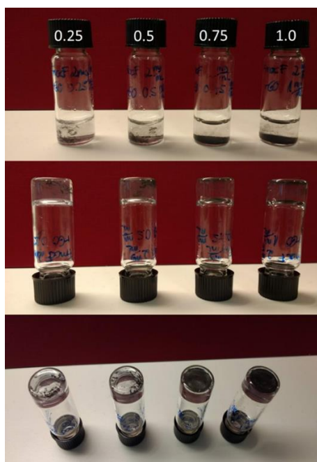
Figure S2. Gelation screening of the Fmoc-F/rGO hybrid system at a range of rGO concentrations (mg/mL). The precipitation of rGO was observed irrespective of its concentration. The concentration of Fmoc-F was constant (2.0 mg/mL).
