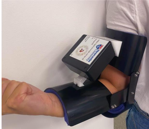
FIGURE 9. Custom at-home isometric resistance training device
