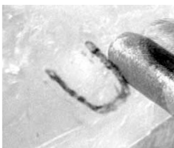
Figure 49. In an “etch-a-sketch” application, the electronic paper is used as a medium for writing text, which can be stored and erased with an opposite voltage, by using a moving pen-shaped top electrode [1].
