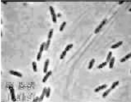
Figure 39. Optical micrograph showing Acetobacter xylinum cells spinning cellulose nanostructures /1/. The dark lines are the cellulose fibrils.
