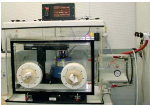
Figure 20. A humidity- and environmental-controlled glove box (PlasLabs) for OLED manufacturing /38/.
