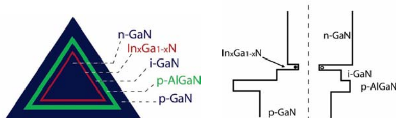
Figure 30. Cross-sectional view of a CMS nanowire structure and the corresponding energy band diagram /65/. The dashed line in the band diagram indicates the position of the Fermi level.
