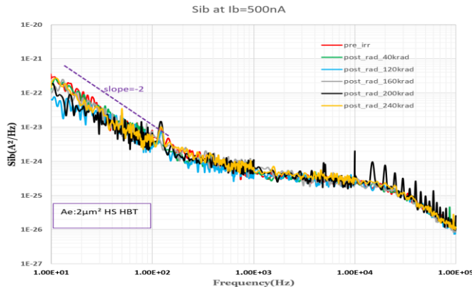
Fig. 34 Sib at I_b=500 \text{ nA} for different irradiation dose on A_e=2 \mu\text{m}^2 HS HBT.
