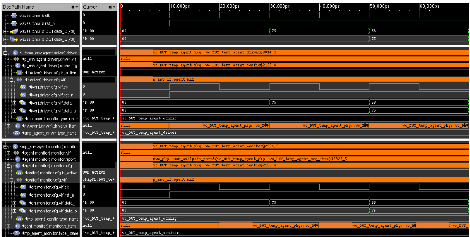
Figure 14: Simulation waveform showing random packets sent to the DUT from the driver and collected in the monitor
