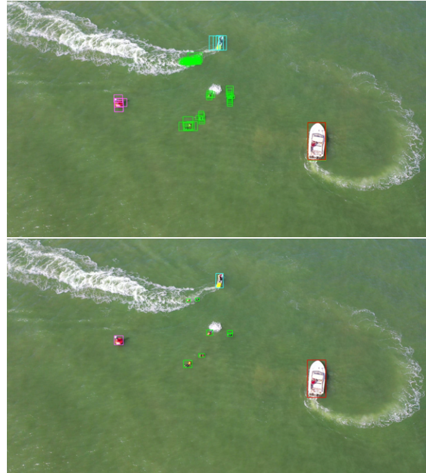
Figure 7: Example predictions from Maritime-VSA (top) and DetectoRS (bottom). Note that we did not filter based on the confidence score, which is why the first method has many predictions for each object. The confidence score for most of them is very low, which is why the AP won't suffer from these.
