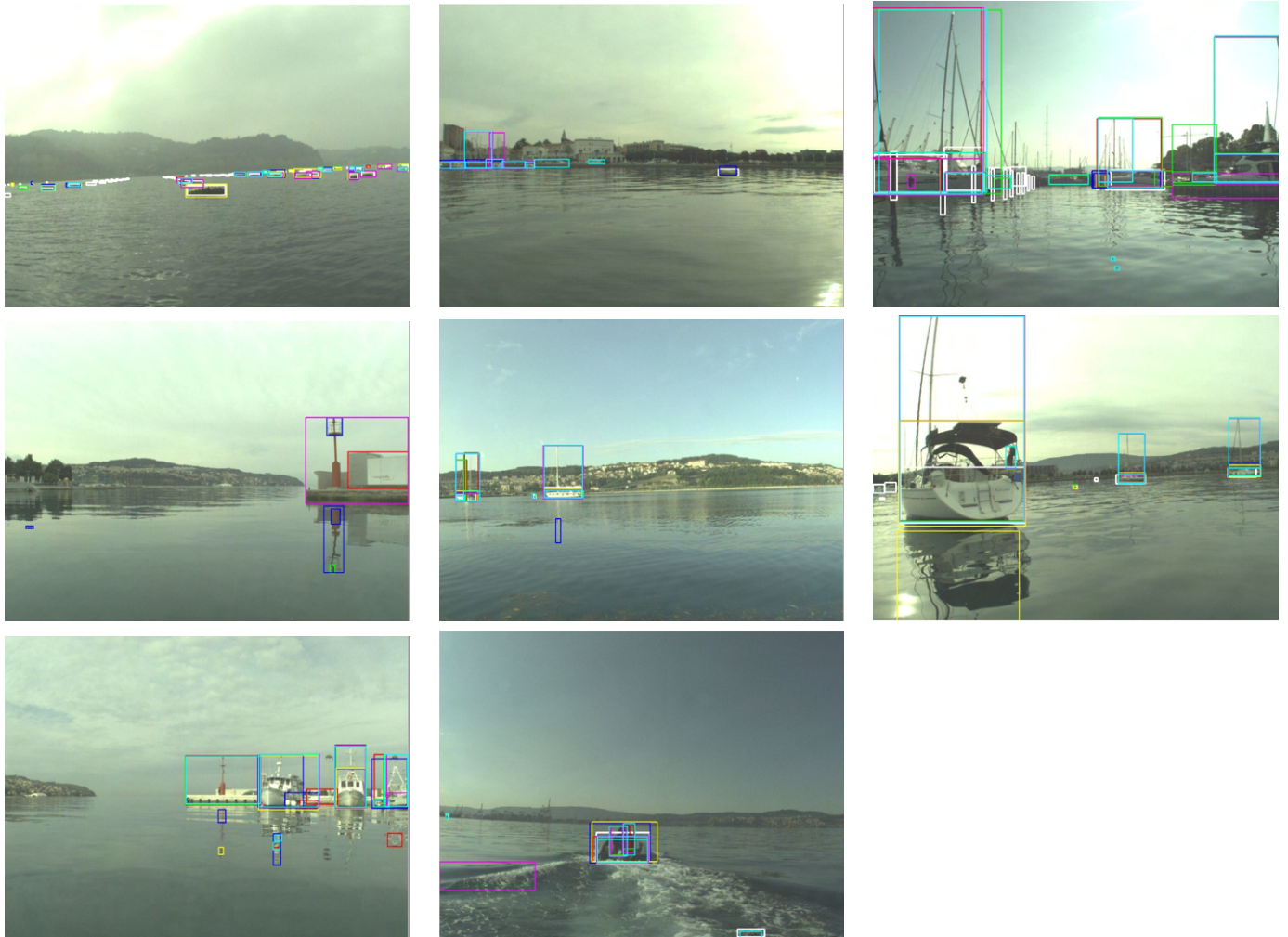
Figure 20: Qualitative comparison of methods for USV obstacle detection. Results of the individual methods are shown with colored bounding boxes as follows: white = ground truth, blue = DetectoRS, red = PRBNet, green = Nvlab x Acvlab’s Yolo v7, yellow = FIOSB KA, cyan = Ocean U, magenta = Nvlab x Acvlab’s PRBNet+Yolo v7.
