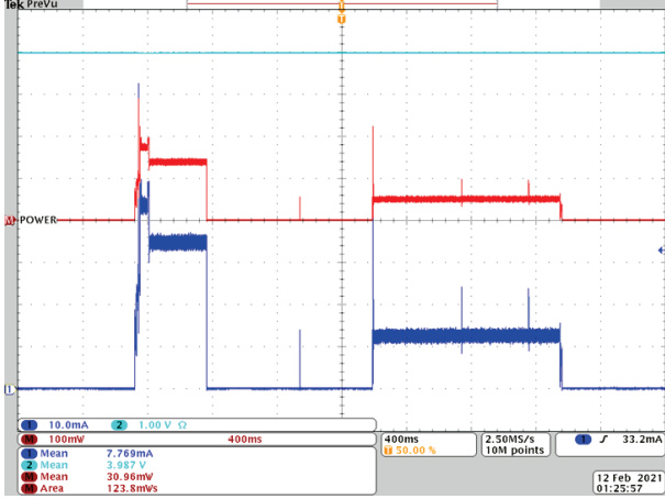
Fig. 3. RT-LRbTC ( N=3 ). Measurement, algorithm and LoRa transmission period with SF10 uplink and SF12 downlink
