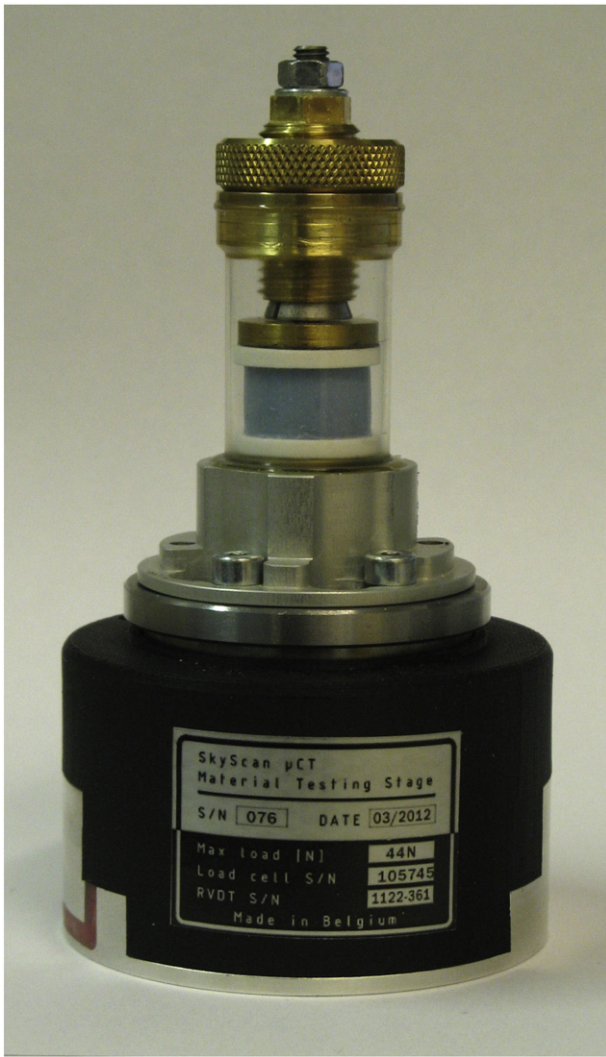
Fig. 4. Sample holder (SkyScan µCT Material Testing Stage) loaded with a rubber test sample used in validating the displacement analysis algorithm.
