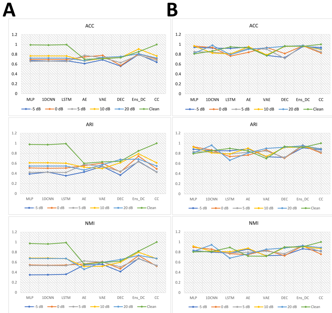
Fig. 6. The performance assessment results, in comparison to the ground truth clustering, for the studied clustering methods from the simulated (left panel) and the real ERP (right panel) data with different additive noise levels. A. the accuracy (ACC), adjusted rand index (ARI), and normalized mutual information (NMI) comparison results for clustering results in the simulated data. B. the performance metrics (ACC, ARI, and NMI) assessment results for the real data. Noticeably, the proposed clustering provides relatively stable and superior results (except when no noise is added) from both applied data.
