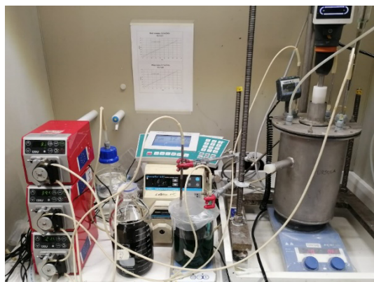
Figure 1. Continuous stirred-tank reactor used for coprecipitation.
