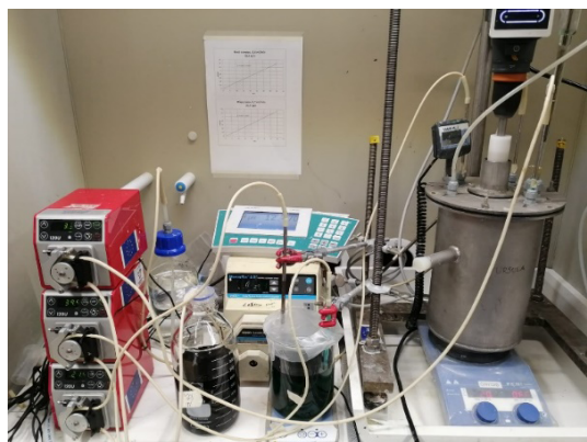
Figure 1. Continuous stirred-tank reactor used for coprecipitation.
