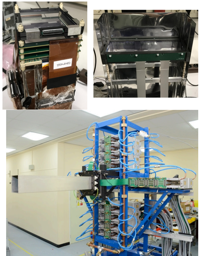
Figure 3: Colour online. Top photograph left: The arrangement of three layers of AIDA DSSD chips in the narrow configuration coupled to one of the \beta Plastic detectors (on top), ready to be inserted into the snout. Top photograph right: AIDA in the wide configuration. Bottom photograph: The built AIDA detector system: the snout on the left contains the several layers of the narrow 8 \times 8 \text{ cm}^2 DSSDs, while the blue frame hosts the electronics. The blue pipes contain the cooling medium for the electronics.
