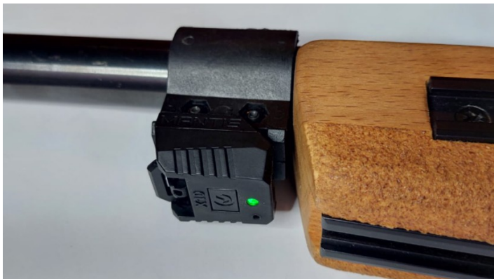
FIGURE 14. Mantis Elite X10 shooting training device attached to a rifle barrel.
