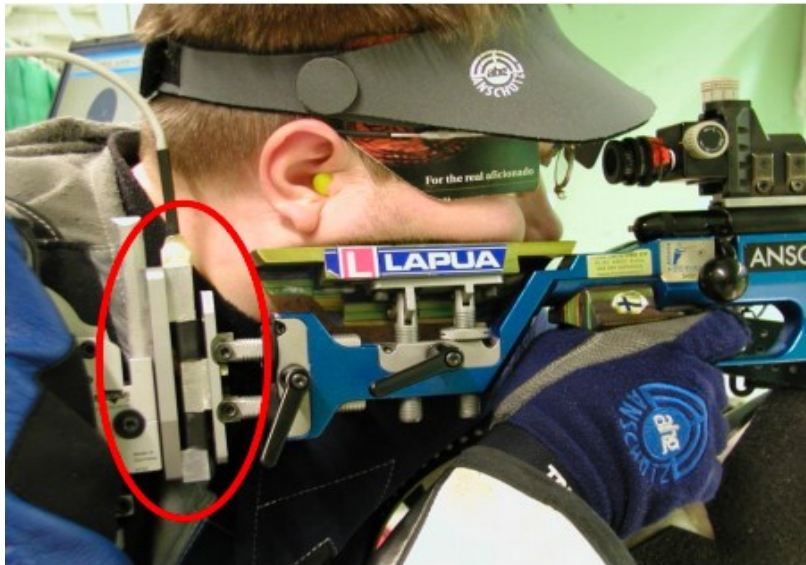
FIGURE 10. The butt section of a rifle with a force sensor attached (Tanskanen, 2013).
