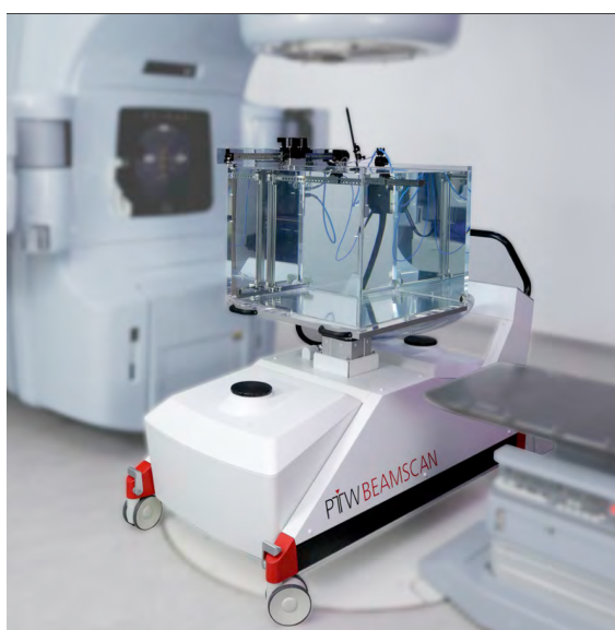
Figure 12. PTW BEAMSCAN water phantom positioned under the treatment machine gantry. [13] During the measurements the phantom was positioned as in the image.
