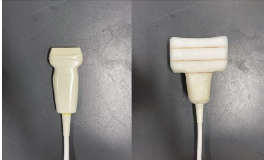
FIGURE 7. Linear ultrasound transducer (60 mm width) used in the study (left) and probe with custom-made probe support used in the VL CSA measurement (right)
