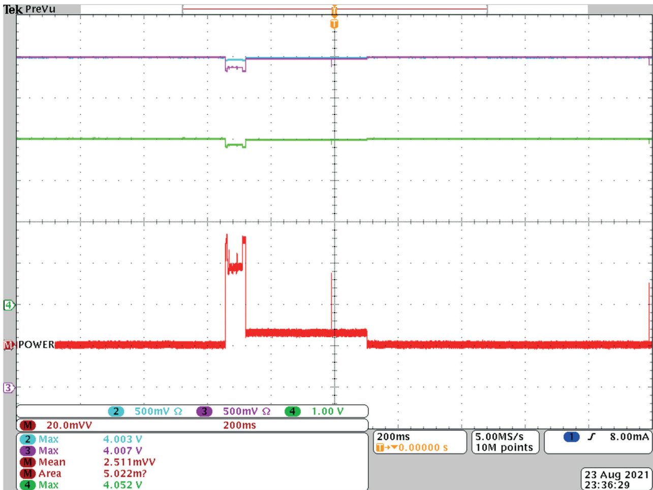
Figure 4 Sensor measurement and data processing energy consumption
