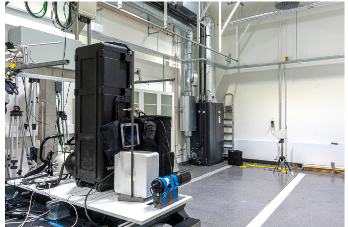
Figure 1: The setup depicting indoor measurements (Indoor II setup) with a moderated ^{252}\text{Cf} source placed on the tripod one meter away from the concrete wall at the back of the calibration hall.
