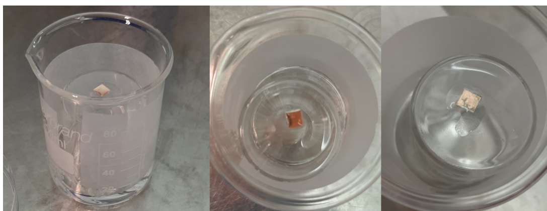
Figure 24: Third experimental attempt. A glass chamber set up without the watch glass. The left and middle figures show the chip covered by the gel immediately after the gel application and the right figure shows the chip and the gel after 24 hours.
