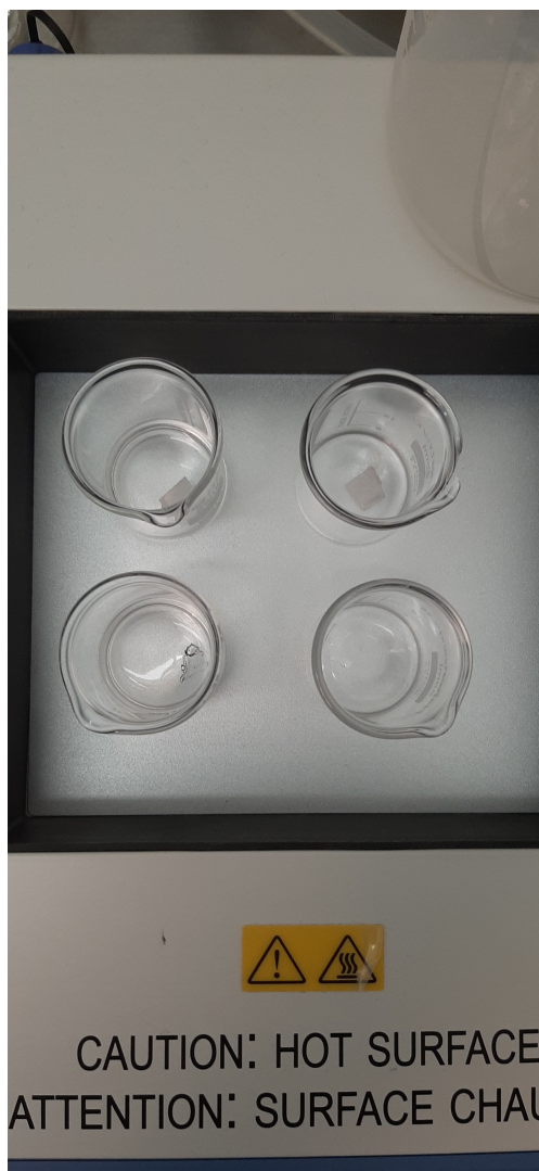
Figure 34: Stability test of the films by heating. HA-anisole film (up) and HA-water film (down). Films heated in water (left) and without water (right).
