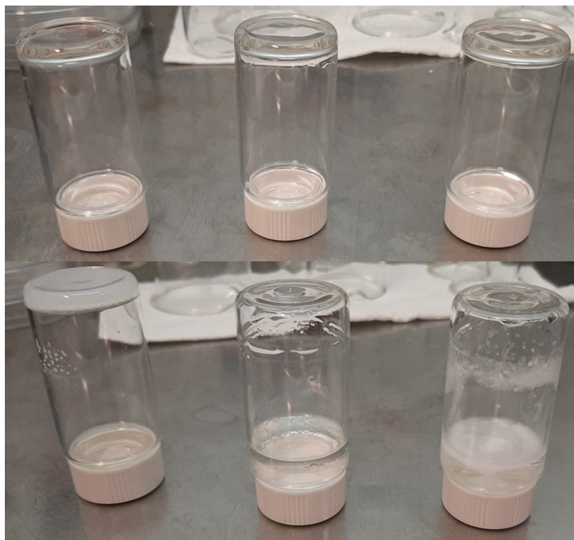
Figure 21: BocFFOtBu gels before (upper) and after (lower) the stability test. Control gel (left), gel tested with water (middle), gel tested with APS (right).
