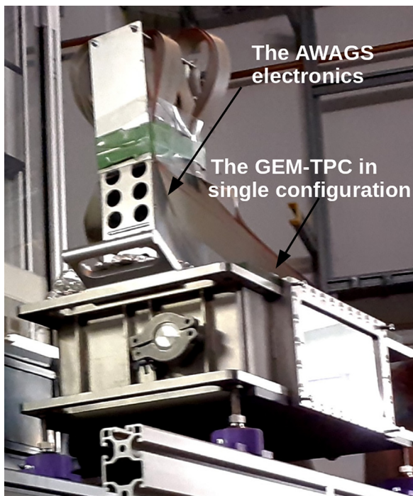
Fig. 3. The HGB4 prototype assembled at the final focal plane of FRS (S4). On the top of the detector under the cover there is the AWAGS electronics.
