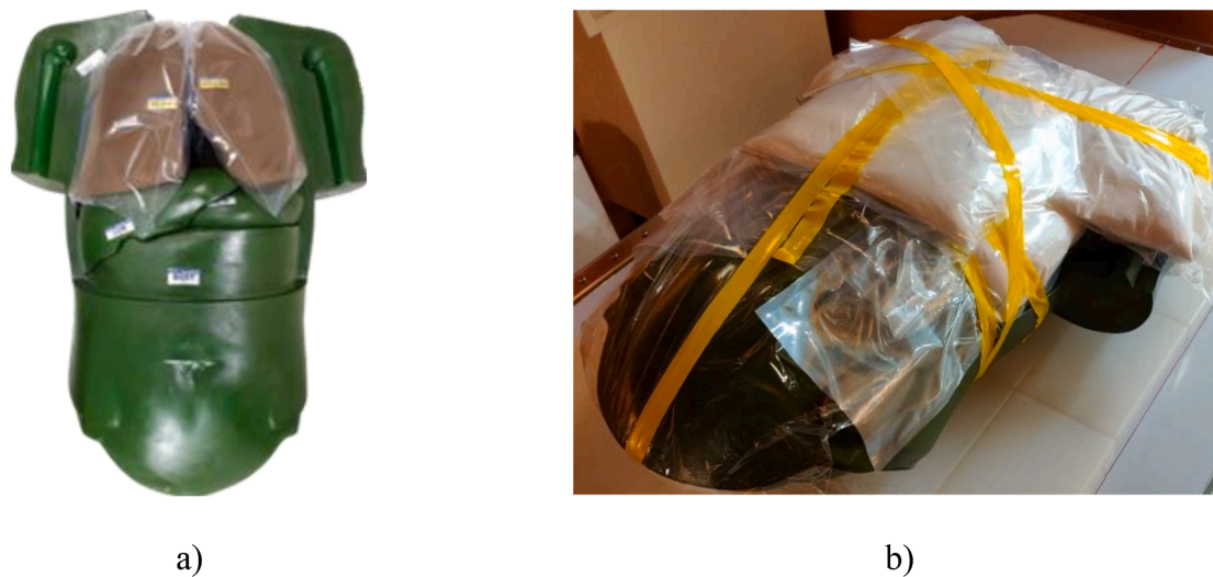
Fig. 1. a) plastic physical phantom (ARDF-09T) without the contaminated chest plate. b) same physical phantom with a custom chest plate made from granulated table sugar.
